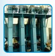
Bucket Elevator to move material in vertical direction and we have taken care of tensioning arrangement and also special design crowned pulley for gripping the bucket belt. We are using casted/fabricated bucket for lift the material. The bucket elevator specially design with rigid construction for its long life.
